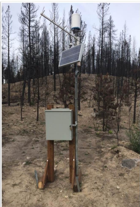
Remote rain monitoring station
