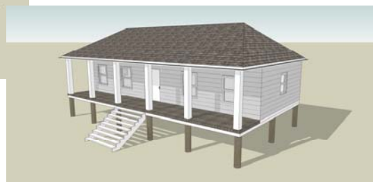
The site shows benefits of "freeboard," raising a coastal house above flood levels. – StormSmartCoasts.org
