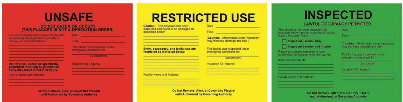
Figure 2 Placards from Applied Technology Council (ATC)-20-1 *Field Manual: Procedures for Postearthquake Safety Evaluation of Buildings, Second Edition* (2005)
